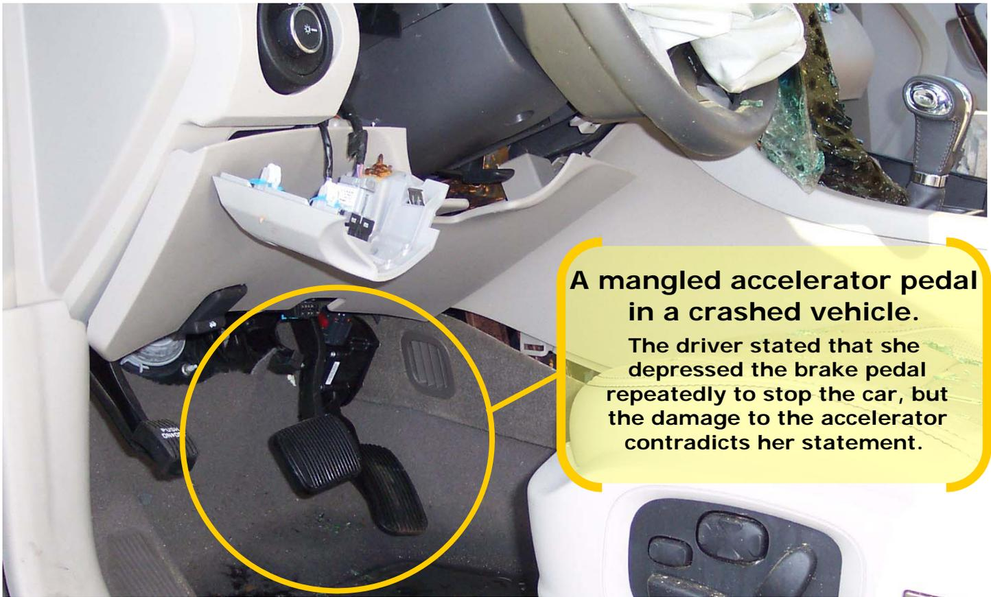
**A mangled accelerator pedal in a crashed vehicle.**
